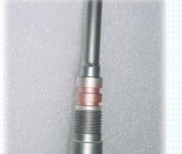
Metal-to-metal vacuum brazing opens up many design possibilities. Often, design features are not conducive to welding. Some combinations of metals, are not weldable. Vacuum brazing allows materials to be joined in a very clean manner with very robust results.
